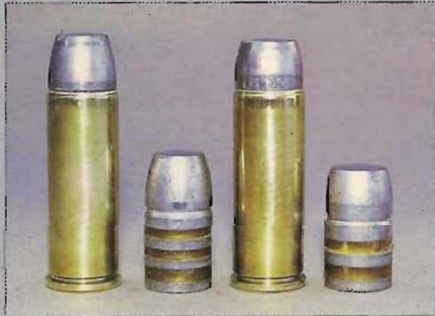
The new Freedom Arms .475 Linebaugh, requires a shorter nose of .360 (right) rather than the .400 length nose (left) originally designed for Linebaugh-converted Rugers.
