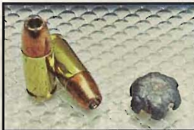
Author's favorite load is 124gr +P+, which expands to 68 caliber and penetrates 12.5".
