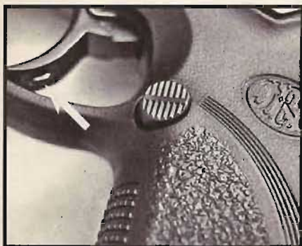
Note trigger has a small over-travel stop.
