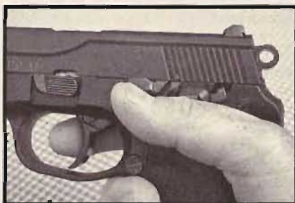
The control levers keep the slide lock lever out of the way of the right hand thumb.
